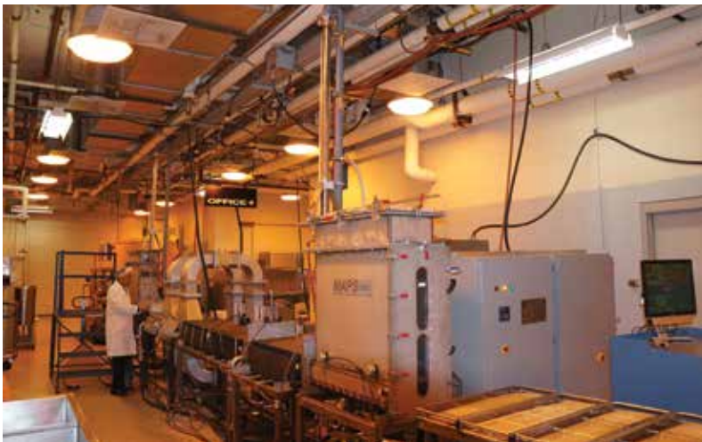
Microwave pasteurizer - A Washington State University-led research team member works on the prototype microwave assisted pasteurization system (MAPS) unit.
