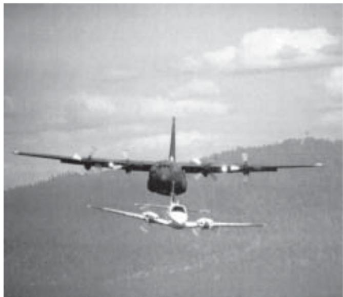
A Beachcraft 58P Baron aircraft that the FS currently uses as a lead plane, guiding an air tanker. FS photo.
