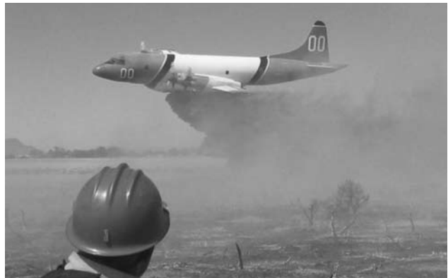
One of the remaining 19 airtankers FS has left under contract (down from 44 in 2002) that will be either too expensive to maintain or no longer airworthy by 2012. The aircraft is a P-3 and is over 45 years old. Zion Helitack, Zion National Park photo.
