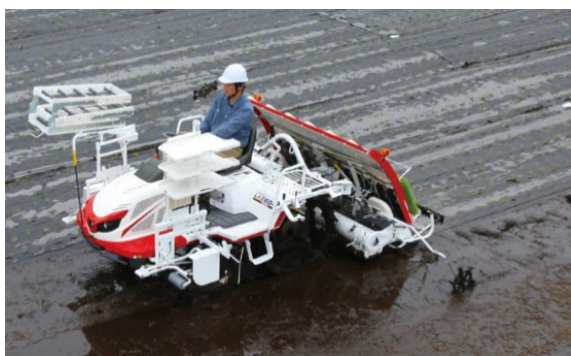
Photo: Rice transplanter using recycled paper mulch
