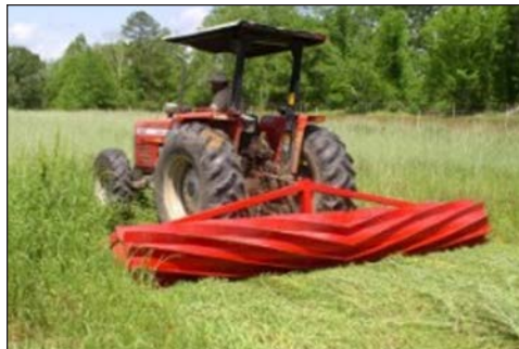
A specially designed roller crimps the rye stem and lays it flat. The next crop is no-tilled into the cover.
