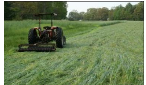
Recycled farm equipment can be used to roll down a rye cover crop. No disking or herbicides is needed.
